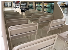
MULTIPLE SEATING IN LIGHTWEIGHT MARINE GRADE ALUMINUM AND MARINE VINYL UPHOLSTERY
