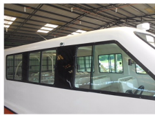
CUSTOM MARINE GRADE ALUMINUM SLIDING WINDOWS WITH TEMPERED GLASS (MADE IN EUROPE)
