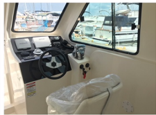
SIDE CONSOLE WITH GARMIN GPS, MARINE VHF, RITCHIE COMPASS AND REMOTE CONTROL SEARCH LIGHT
